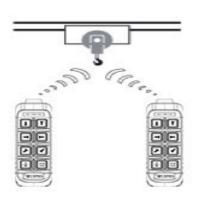
Allow two or more operators to be equipped with one transmitter independently and use the same crane independently. The "takeover release" is independent of each other and does not interfere with each other.
