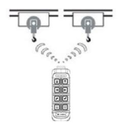
Using a one-to-two function one transmitter can control two cranes and the control of each crane can be selected through the button switch on the transmitter.
